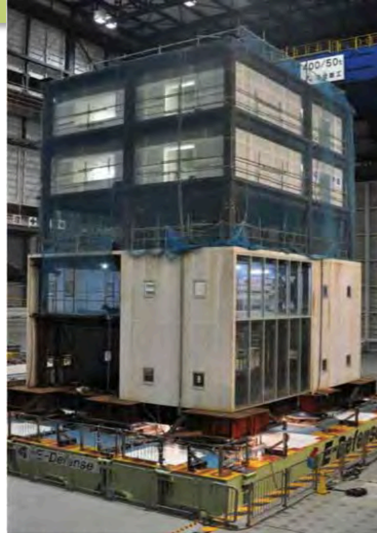
At E-Defense, shake table tests were performed on a 5-story full scale steel moment frame building isolated with triple pendulum bearings. The isolation system consisted of 9 bearings, one beneath each column of the building.
